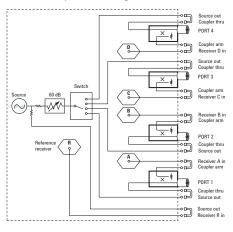
4-port configurable test set, extended power range and internal second source
