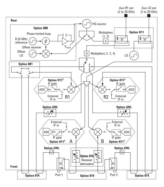
Option H11: IF-gate controls and external-IF inputs are accessed on rear panel.
